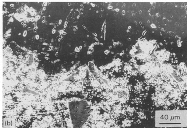
Figure 4 Metallographic observations on the area segregated with tungsten particles in Sample III, through (a) OM, and (b) SEM.
